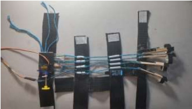
Figure 1: Shows the exoskeleton portion of the device. It includes the servo and vibration sensor.
