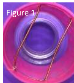
Figure 1 illustrates how the copper wires were inserted through the middle of the bottle.
